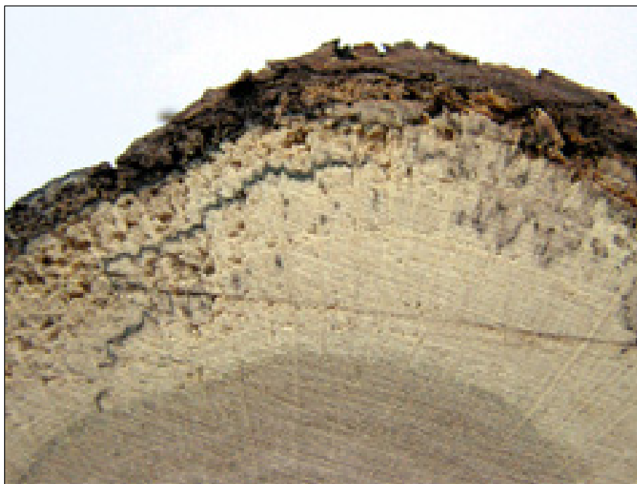
Fig. 11: The decayed wood are often accompanied with black zone lines in the sapwood.
