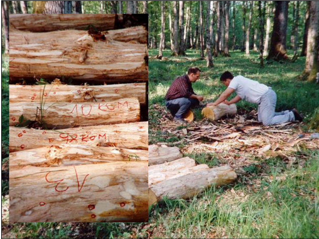
Fig. 4: Debarbing at the end of the exposal period (insert shows counted and marked pinholes on oak logs of the control group).
