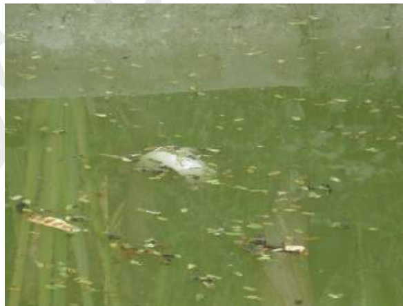
A moss bag in monitor metal content in water (Source: Govindaparyari et al. 2019)
