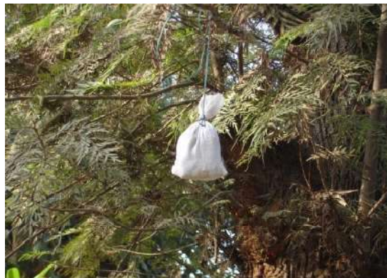
A moss bag to monitor the air metal contents of the site (Source: Govindaparyi et al. 2019)
