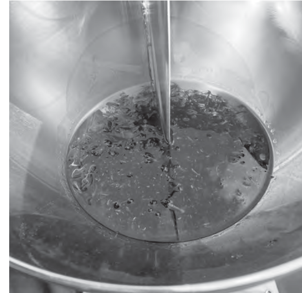
Fig. 3. The insect sample fractionizer in action. Axial rotation distributes the invertebrates in the total volume into equally sized parts.
