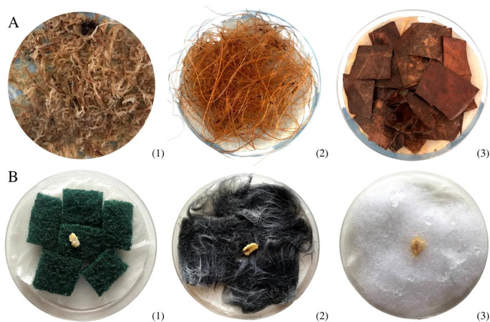
Figure 2. Substrates utilized in the experiment: [A] Natural: (1) dried sphagnum moss, (2) coconut coir fiber, (3) leaf litter, and [B] Synthetic: (1) scouring pad, (2) faux fur cloth, and (3) polyester fiber.
