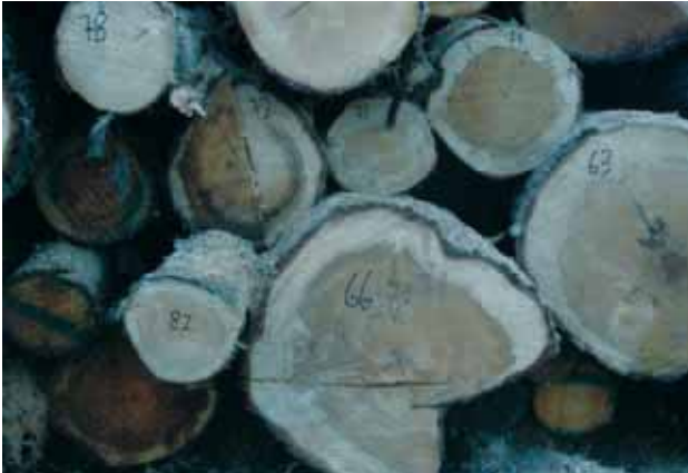
Fig. 18. Part of a pile with rotten log ends. C. borealis was isolated from log no. 63; H. parviporum was isolated from logs no. 72 and 78; P. chrysoloma was isolated from logs no. 71, 74 and 82; S. sanguinolentum was isolated from log no. 66. Photo: H. Solheim
