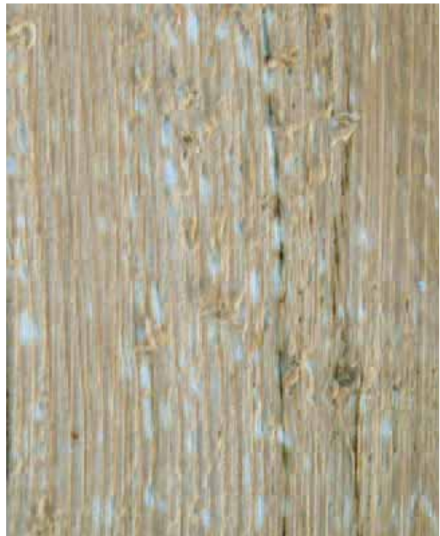
Fig. 13. A longitudinal cut of P. chrysoloma rot with the characteristic white, rather large pockets. Photo: H. Solheim
