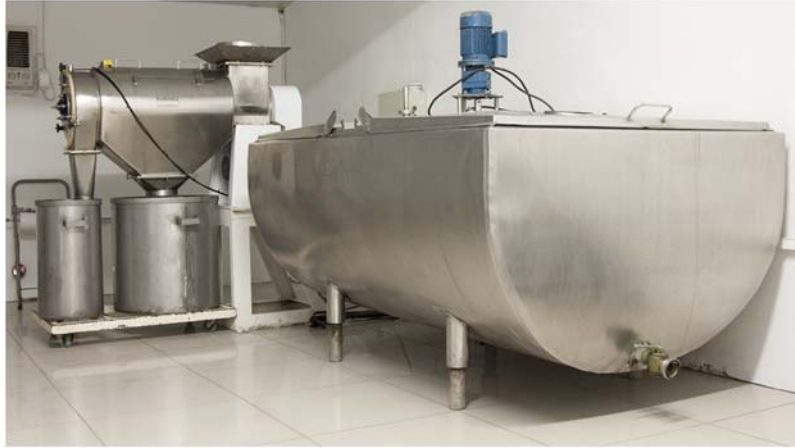
FIGURE 15.8 Modern baculovirus processing equipment, homogeniser, filter and bulk temperature-controlled storage of baculovirus suspension.
