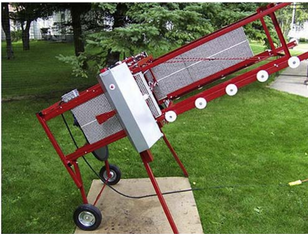
FIGURE 19.3 An alfalfa leafcutting bee cocoon extractor. This Dual Pinmatic Harvester is capable of harvesting 420 nests per minute (PINMATIC Inc., Pinawa, Manitoba). For color version of this figure, the reader is referred to the online version of this book.
