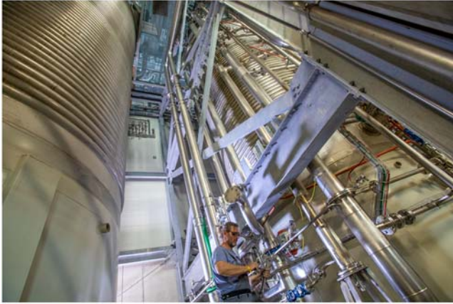
FIGURE 12.1 Large scale fermenter vessels at E-Nema GmbH, Schwentimental, Germany. Photo Dr Arne Peters.
