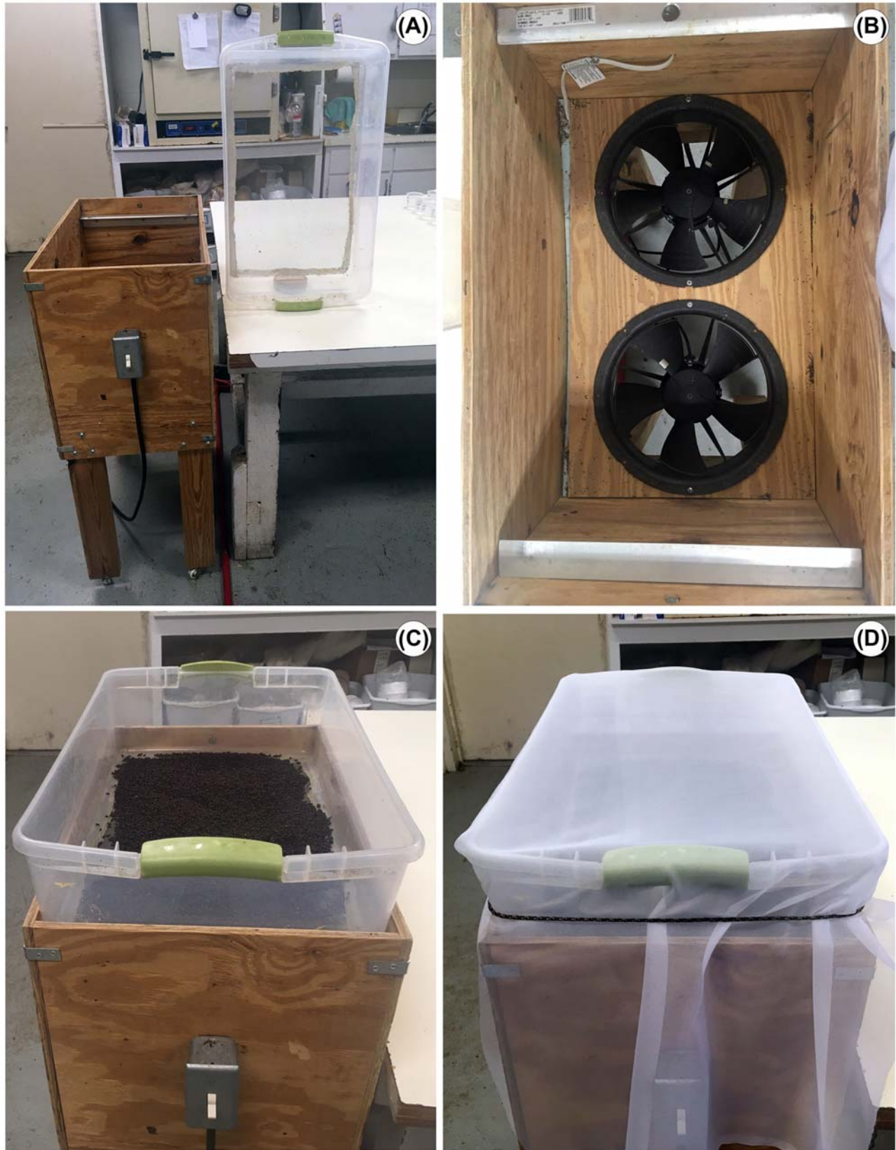
FIGURE 5.11 Device for drying fly pupae after separating from media by floatation. (A) The drying box is constructed from plywood with an attached power supply and plastic containers with screen mesh bottoms are fitted inside the box. (B) Inside the box, two fans pull air through the top of the box and vent through the underside. (C) Wet pupae are placed in containers and covered with fine mesh screening (D) to prevent stray parasitoids from reaching the pupae.
