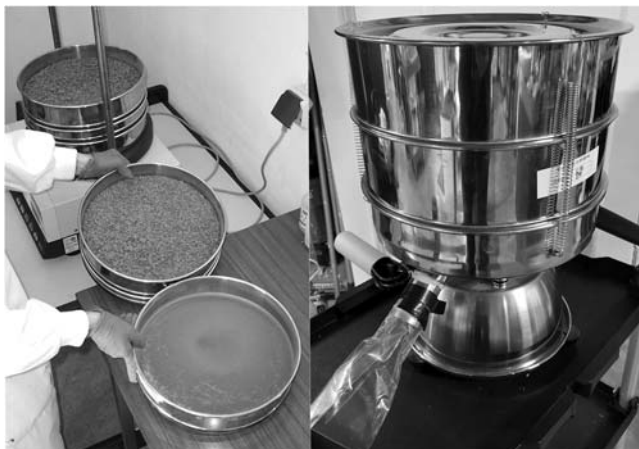
FIGURE 11.6 (Left) Batch harvesting conidia of Metarhizium anisopliae from substrate by mechanical classification using 20- and 100-mesh sieves on a vibratory shaker. (Right) Electric, vibratory, powder separator, made for domestic kitchen use but ideal for the small-scale harvest of conidia from the solid substrate, can process 1 kg of dried substrate per 15-minute cycle in the author's laboratory. A 33-cm diameter, 10- or 20-mesh sieve is fitted above an 80- or 100-mesh sieve mounted above a collecting pan. Conidia are collected through the spout at the lower left into a sealed container (plastic bag shown).
