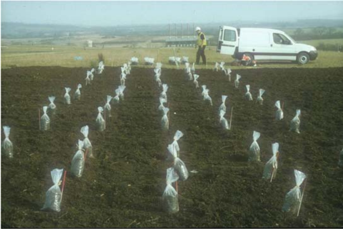
FIGURE 21.2 Two-liter EIUs transported to an organic matter enriched landfill cap postcultivation phase. The plastic envelopes, tied at the neck, are removed prior to soil-inoculation.
