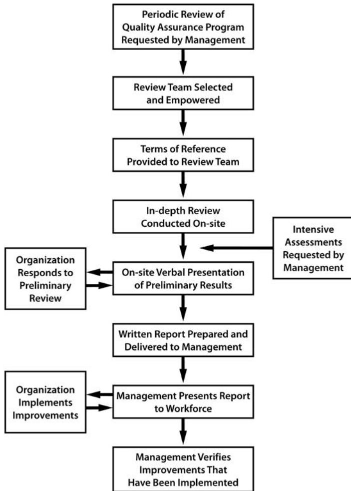
FIGURE 9.4 Process for reviewing a quality assurance system for arthropod mass production based on the experience of the author and Juran et al. (1979).
