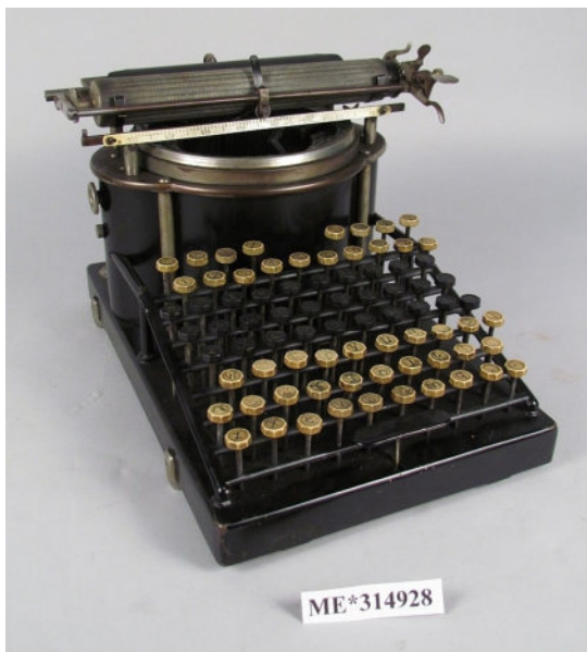
Fig 8. Collin's Yost typewriter; note the separate keyboards for capitals and lowercase letters.
