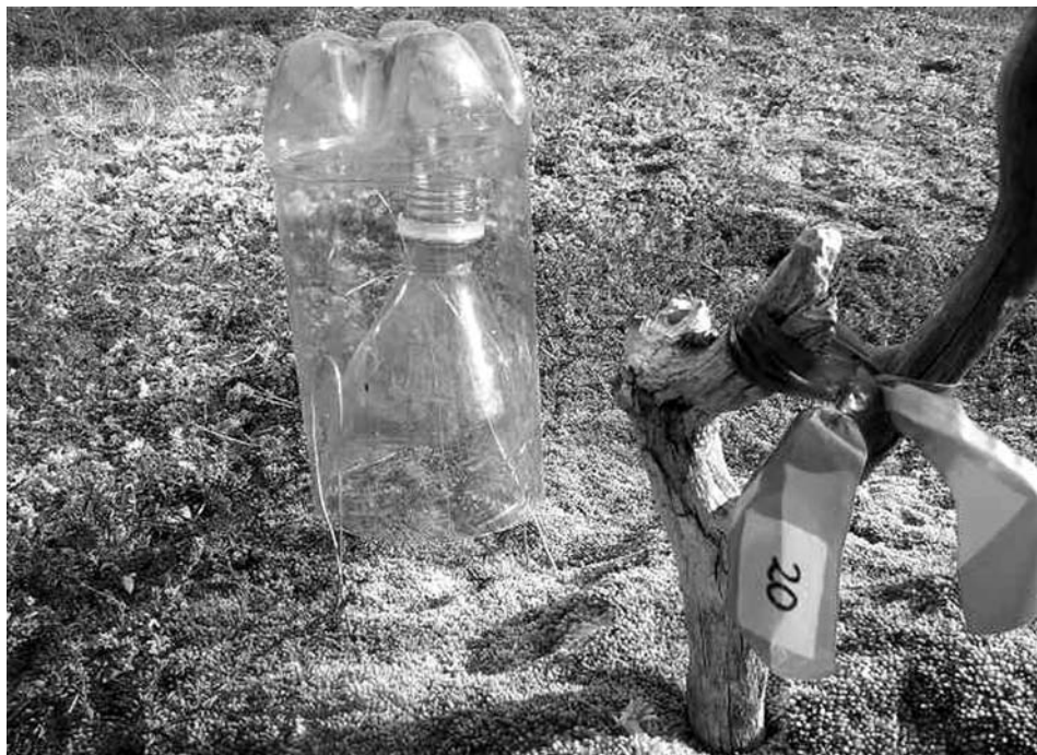
Fig. 3. Model of the trap used to catch flies that visited sporophytes of Tayloria dubyi . This trap was constructed using recycled 1 litre plastic bottles.
