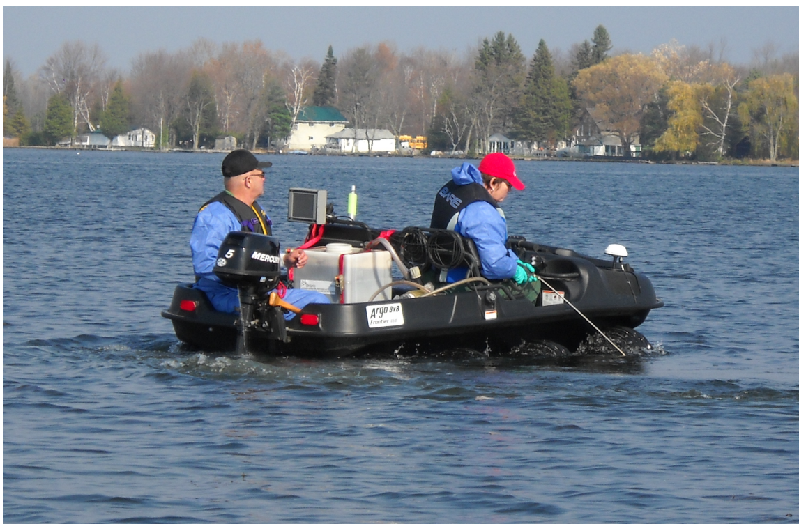
Figure 20: John Graham Agro-Services/ Port Britain Chemical performing fall 2012 Diquat application. Using an amphibious vehicle (Argo 6x6) they are able to traverse the debris filled waters of the Trent River. The chemical was applied with a long, extendable wand to maximize plant-chemical contact
