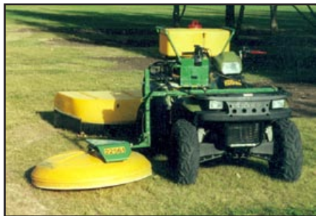
Photo 7-8: The Enviromist® sprayer mounted on an ATV at the PFRA Shelterbelt Centre in Indian Head (SK).
