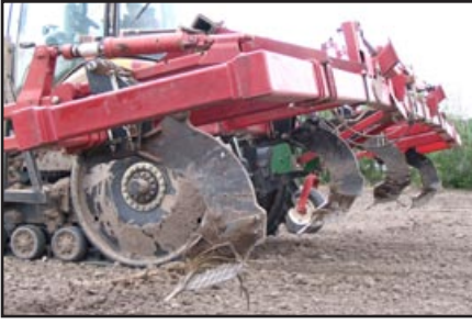
Photo 6-7: Marking with a '4-row' row marker at one of AL-PAC's farms in Alberta. The tractor is a Cat Challenger (200 hp) with a GPS system hooked up to an auto-steer system. This allows the tractor to stay on course both ways. The 4 subsoilers mounted on the toolbar are at 3.0 m (10 ft.) spacing.
