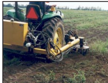
Photo 7-17: The operator controls the movement of the rotating tiller. This machine is actually working an R-1 crop at one of Alberta-Pacific Forest Industries Inc.’s poplar farms near Boyle (AB). Due to the small tree size, the operator controls the movement of the rotary tiller.
