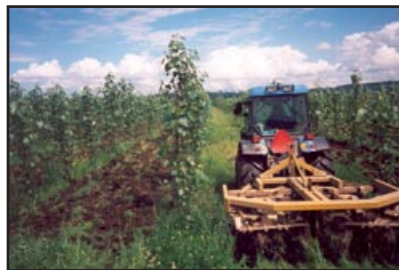
Photo 7-13: Offset tandem disk used with a small orchard tractor (about 80 hp) to break up the weed growth in a poplar crop near Snohomish (WA). This disk is about 2.4 m (8 ft.) wide.
