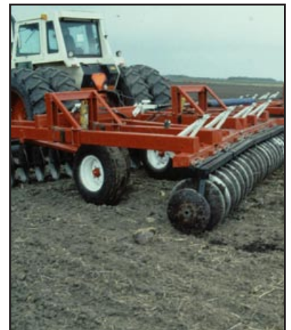
Photo 5-2: A tandem disk used as a cultivating disk for a secondary cultivation.
