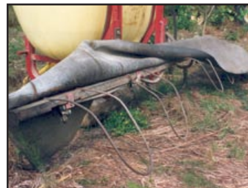
Photo 7-7: Shielded sprayer for use inside a poplar crop in Ontario. A real simple, cheap but effective shield for application of glyphosate-based herbicides.
