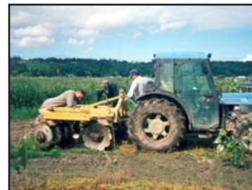
Photo 7-14: Offset tandem disk used with a small Landini orchard tractor (about 80 hp). This unit is very compact and the features of the orchard tractor make it very maneuverable.
