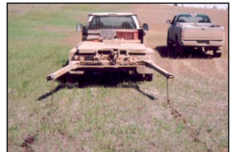
Photo 6-4: A very simple marker attached to the bumper of a flatbed truck 'scratching' tree row locations on a field in 2004 near Maidstone (SK).
