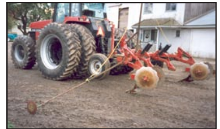
Photo 6-5: This ‘2-row’ row marker was used in Whatcom County in Washington State. It clearly shows the two subsoiler shanks. Also visible is the marker in the bottom left corner that marks a line for the return trip.
