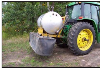
Photo 7-6: Shielded sprayer for use inside a poplar crop in Minnesota.
