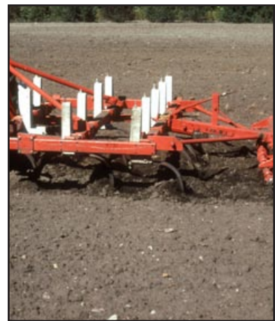
Photo 5-5: Cultivator with mounted harrows on a farm in Saskatchewan.
