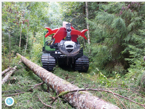
Removal of timber using an appropriate skidder
