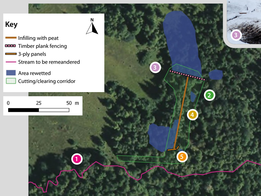
Plan showing the works conducted as part of the restoration of the Crossat peatland
